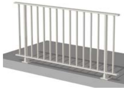
Vertical rails beneath handrail
