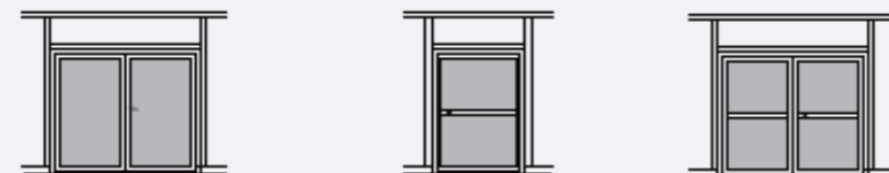
2-leaf door, pocket glazing with handle 1-leaf door, pocket glazing with knob 2-leaf door, pocket glazing with knob
