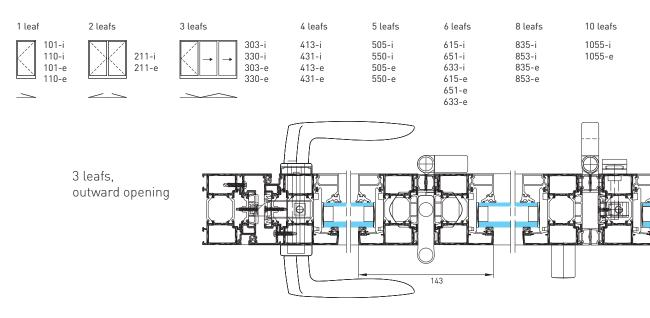
From 1 to 10 leaves, inward or outward opening with identical configuration
