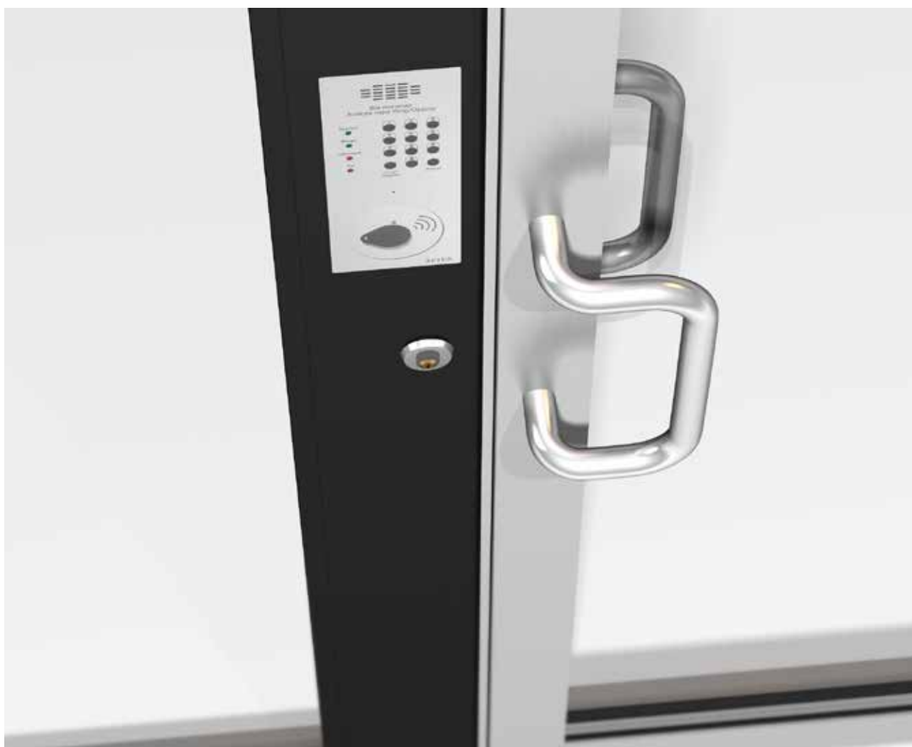
Entrance with entry phone/access control system. Door in natural anodised finish with powder coated frames. Lock installed in frame. Reinforced rebate section.
