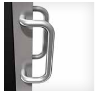
Offset handle with concealed attachments. Height 300 mm, Ø 30 mm. Aluminum.
