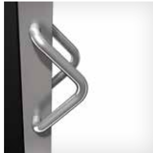
Triangular handle with concealed attachments. Height 300 mm, Ø 30 mm. Aluminum.
